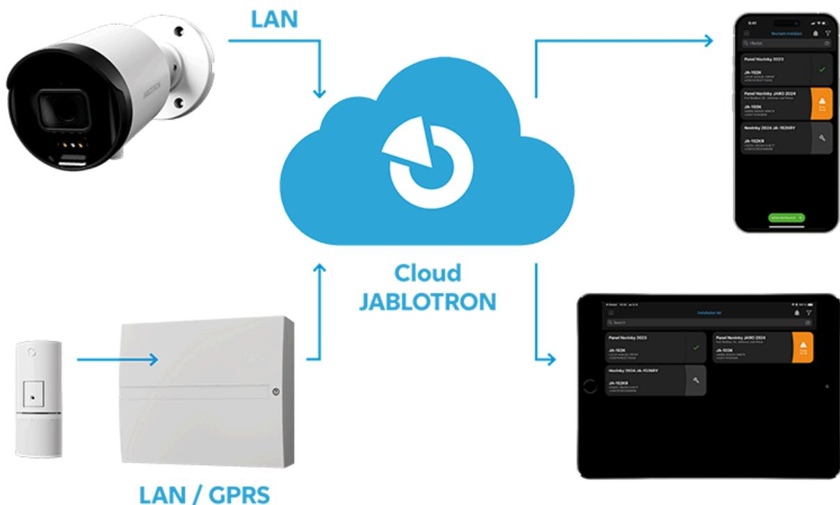
*Fig. 2: Diagram of JABLOTRON CLOUD functioning*
