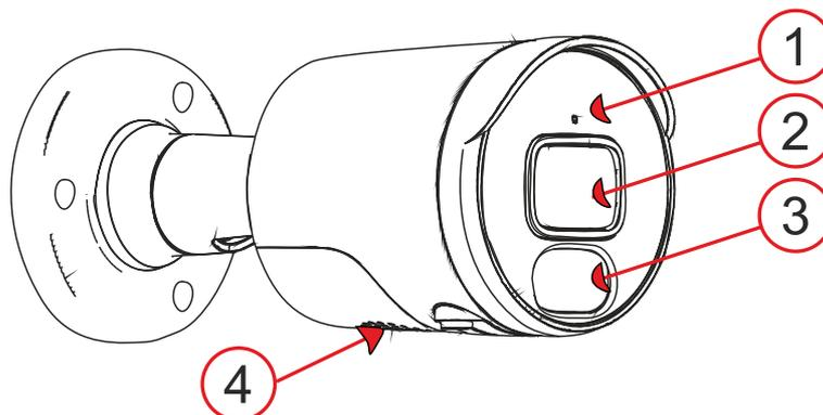
*Fig. 1: Description of the external parts of the product*
