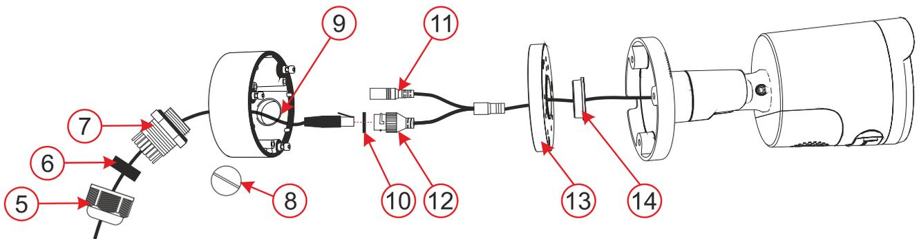
*Fig. 3: Installation procedure using the mounting socket*
